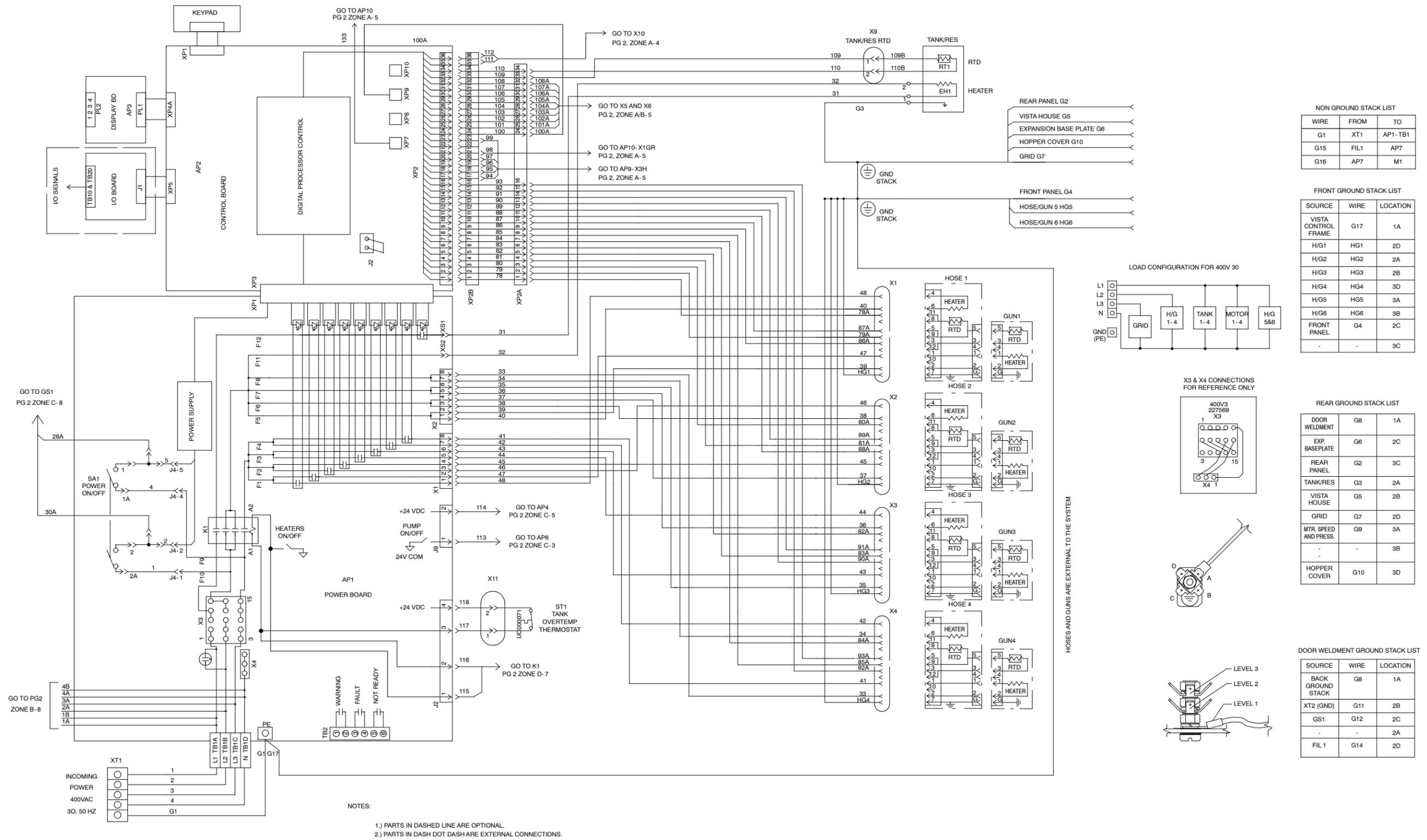
Fig. A 8-4 FoamMelt 200 Processor Wiring Diagram: 400 Volt (page 2 of 2)
